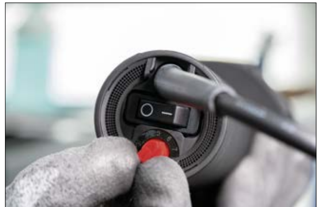
Adjusting H6100 operation temperature.
